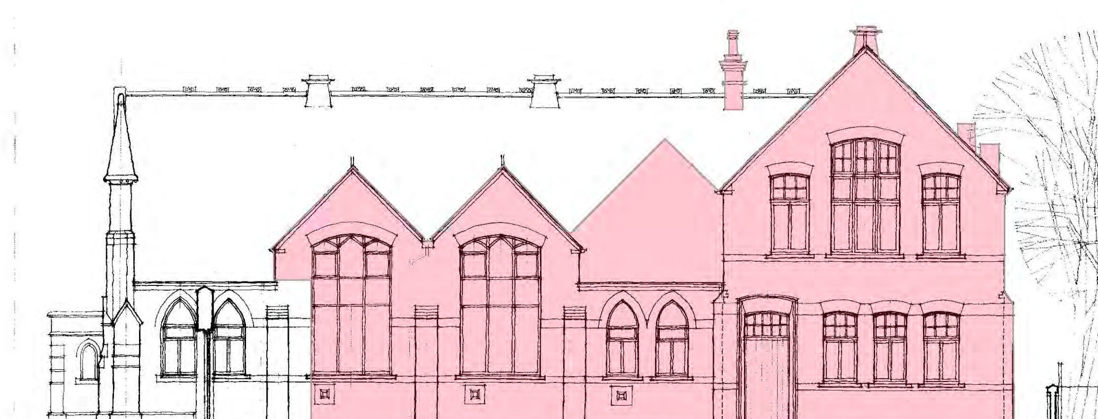
Demolitions Hall East Elevation
